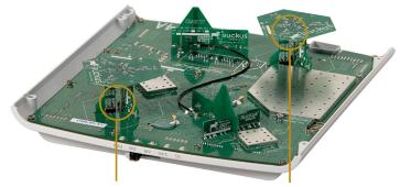
BeamFlex+ Adaptive Antenna Technology
